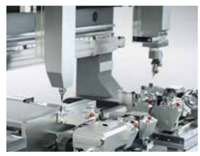
Working areas Depending on the machine concept, varies between 1000 mm and 2200 mm width
