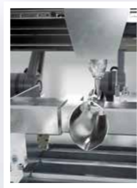
Laser cutting of the hole
