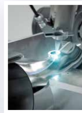
Laser welding of the threaded bushing
