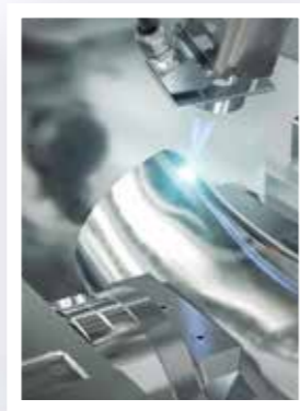
Welding of the half shells with laser
