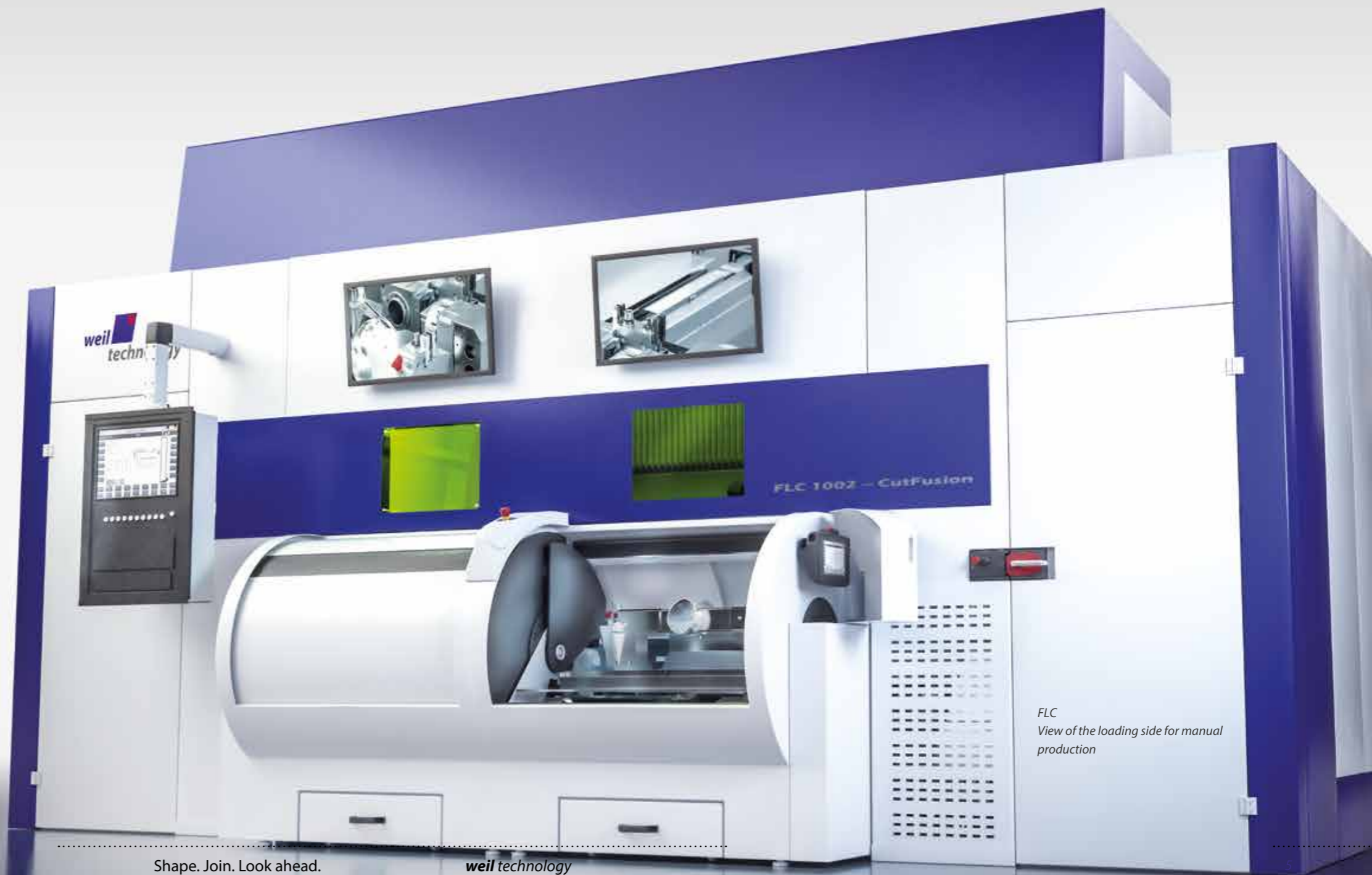
Working areas Depending on the machine concept, varies between 1000 mm and 2200 mm width
