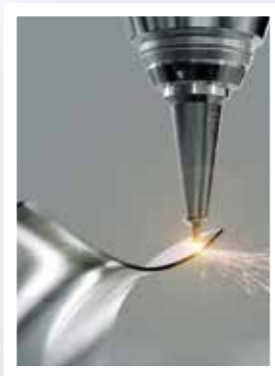
Laser trimming of the half shells
